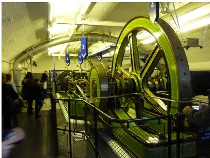
One of the original steam engines that powered Tower Bridge
