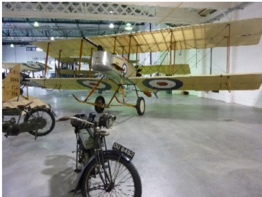
Two-seater pusher military biplane of WWI - Vickers FB 5 Gun Bus with a propeller at the rear, see page 6.
